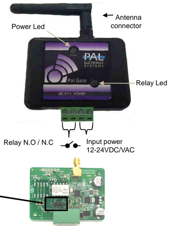
There is an option to change the relay mode using the N / O / N.C.
